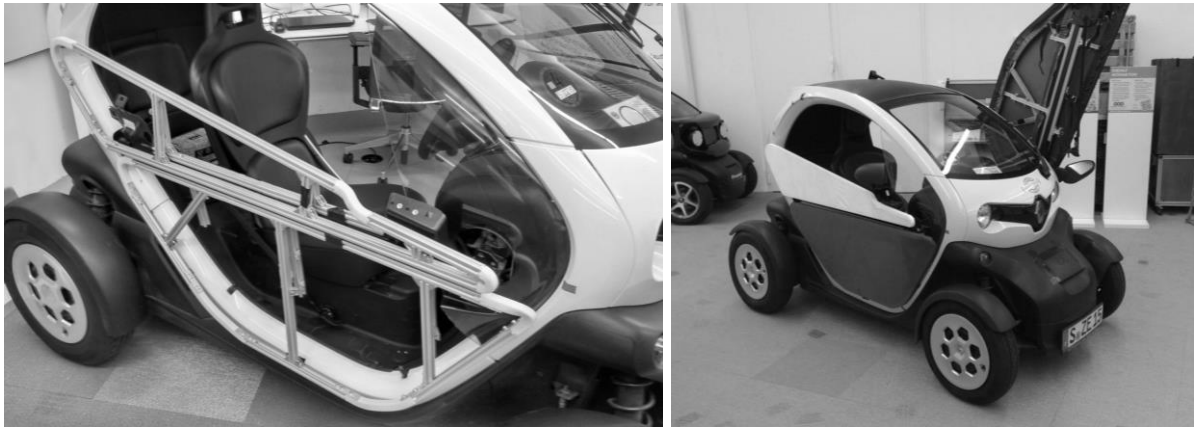
Figure 7: Left: Demonstrator with aluminium frame. Right: Finalized Demonstrator with textile doors.
