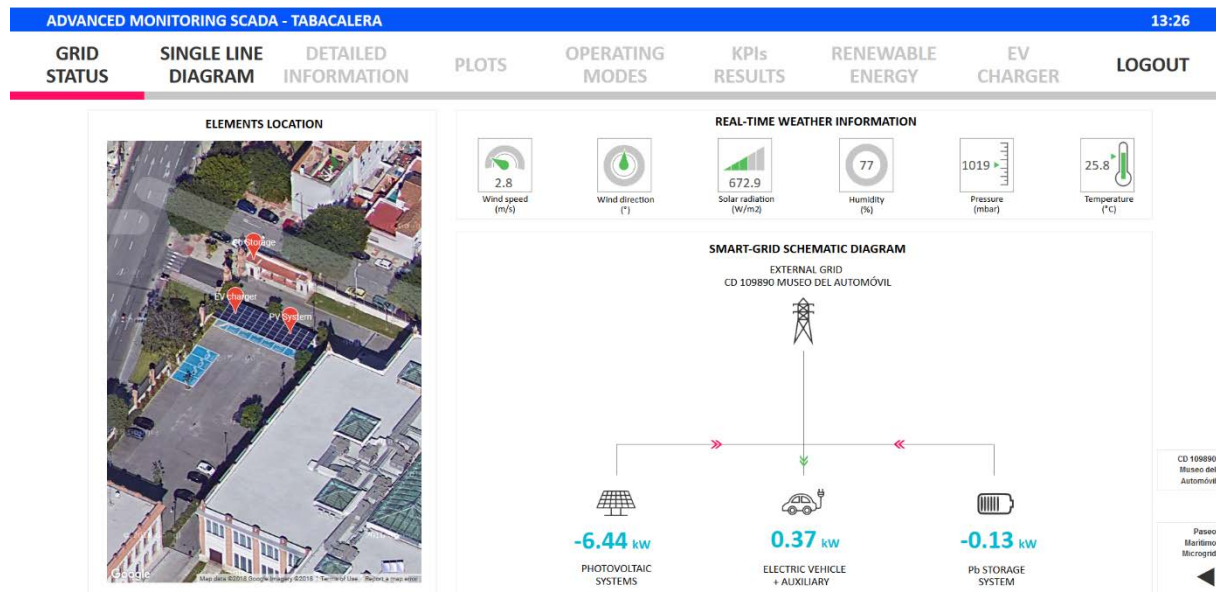
Figure 7. Example of SCADA main page: Grid Status.
